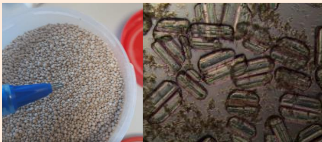
Figure 18. Struvite harvested and struvite under microscope from crystallization process
